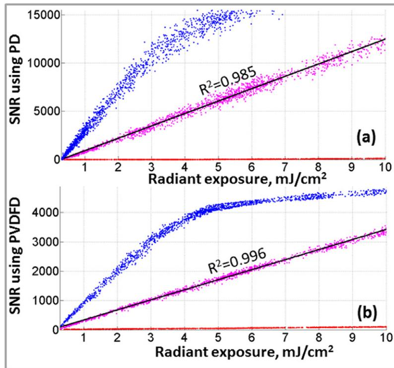
**Figure 3.** (a), (b) The DR SNRs measured using the PVDFD or PD in three phantoms: (red)—distilled water; (magenta)—0.15% aqueous solution of lipofundin; (blue)—1.5% aqueous solution of lipofundin; (black)—linear fit to experimental data.
