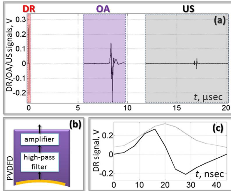
**Figure 2.** Triple-modality measurements using the OA detector. (a) Sample A-scan with DR/OA/US signals. (b) Spherically-focused PVDFD used for the measurements. (c) Band-limited sample DR signal (solid line) and its envelope (dotted line).
