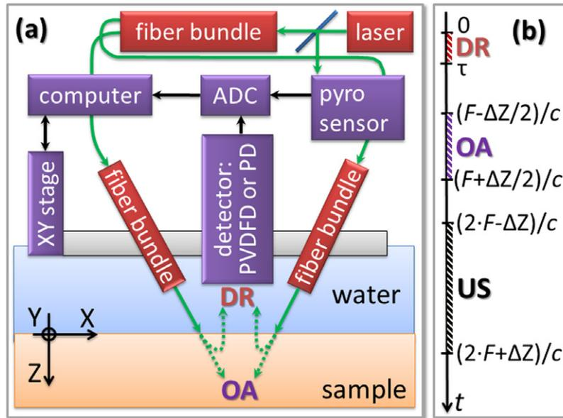
**Figure 1.** The experimental setup for OA/US/DR imaging. (a) Schematic of the experimental setup: photons absorbed by the sample generate OA signals, while photons absorbed by OA detector generate the measurable DR signal as well as providing the probing US pulse. (b) Sketch of the information contained in an A-scan with the sequence of the DR, OA, and US signals.
